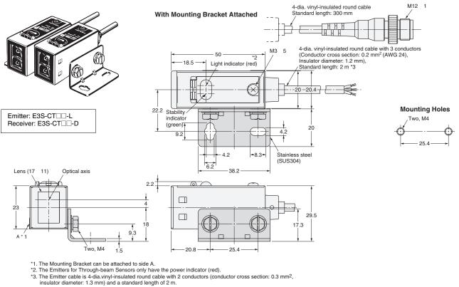
Note: Models numbers for Through-beam Sensors (E3S-CT11(-M1J)) are for sets that include both the Emitter and Receiver. The model number of the Emitter is expressed by adding "-L" to the set model number (example: E3S-CT11-L 2M), the model number of the Receiver, by adding "-D" (example: E3S-CT11-D 2M.) Refer to Ordering Information to confirm model numbers for Emitter and Receivers.
