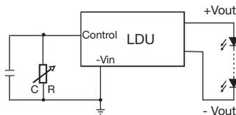
Shorting out the Control pin to GND will turn the output off.
