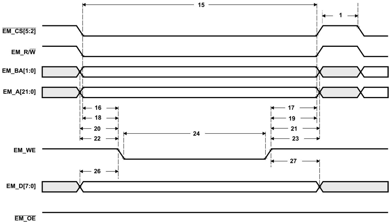
Figure 6-15. Asynchronous Memory Write Timing for EMIF
