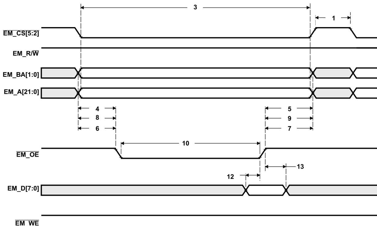
**Figure 6-14. Asynchronous Memory Read Timing for EMIF**
