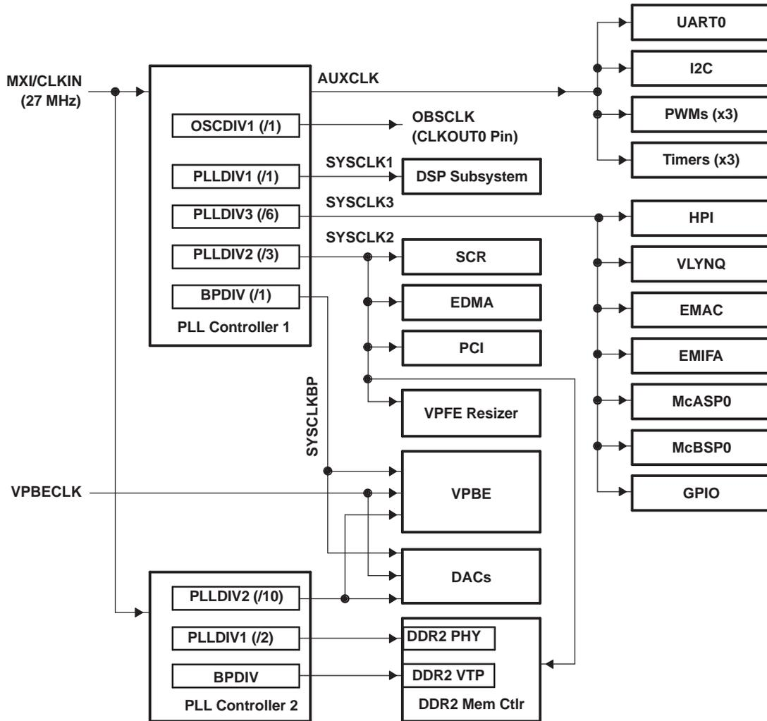
Figure 6-4. PLL1 and PLL2 Clock Domain Block Diagram
