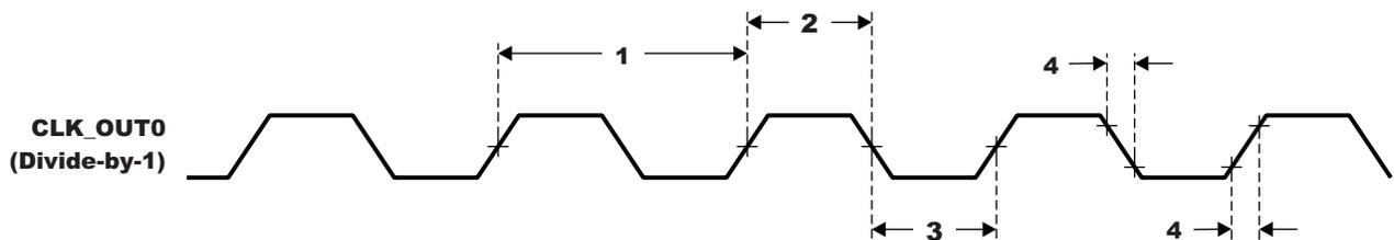
Figure 6-13. CLKOUT0 Timing
