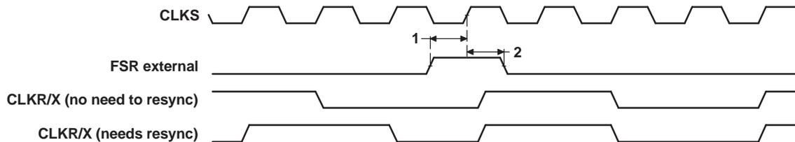
Figure 6-31. FSR Timing When GSYNC = 1
