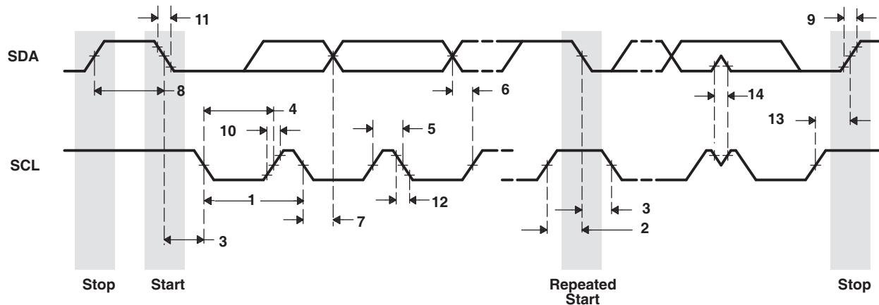
**Figure 6-26. I<sup>2</sup>C Receive Timings**
