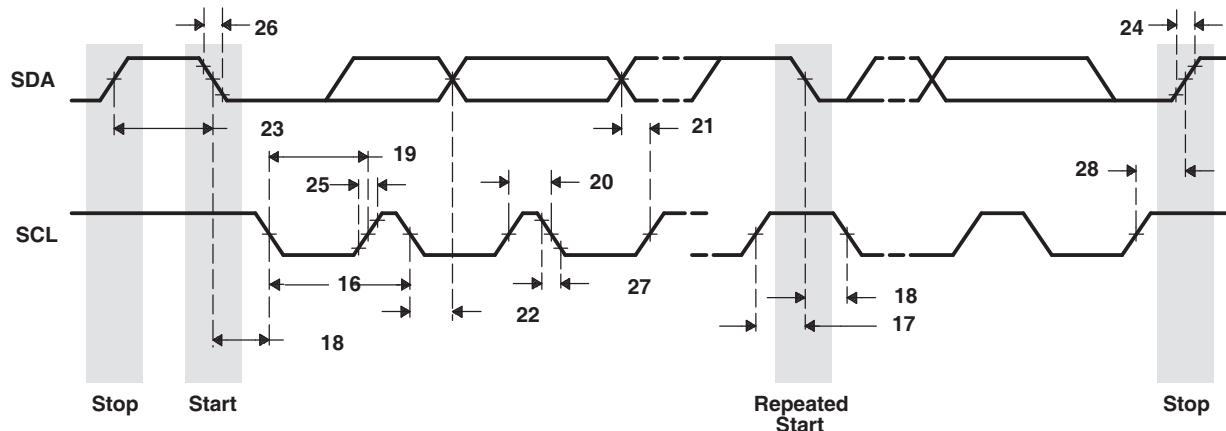
**Figure 6-27. I<sub>2</sub>C Transmit Timings**
