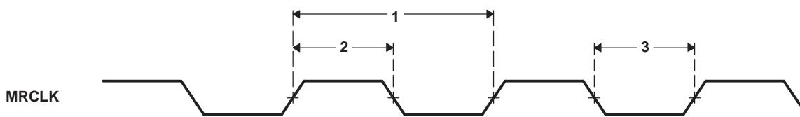
**Figure 6-39. MRCLK Timing (EMAC - Receive)**
