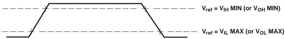
**Figure 6-3. Rise and Fall Transition Time Voltage Reference Levels**
