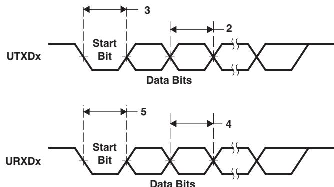
**Figure 6-24. UART Transmit/Receive Timing**
