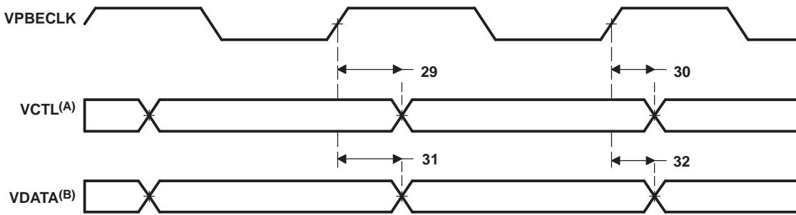
A. VCTL = HSYNC, VSYNC, LCD\_FIELD, and LCD\_OE
