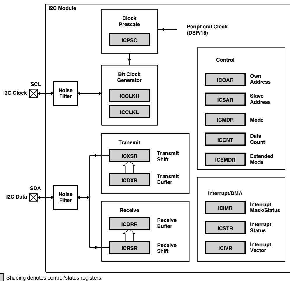
**Figure 6-25. I2C Module Block Diagram**
