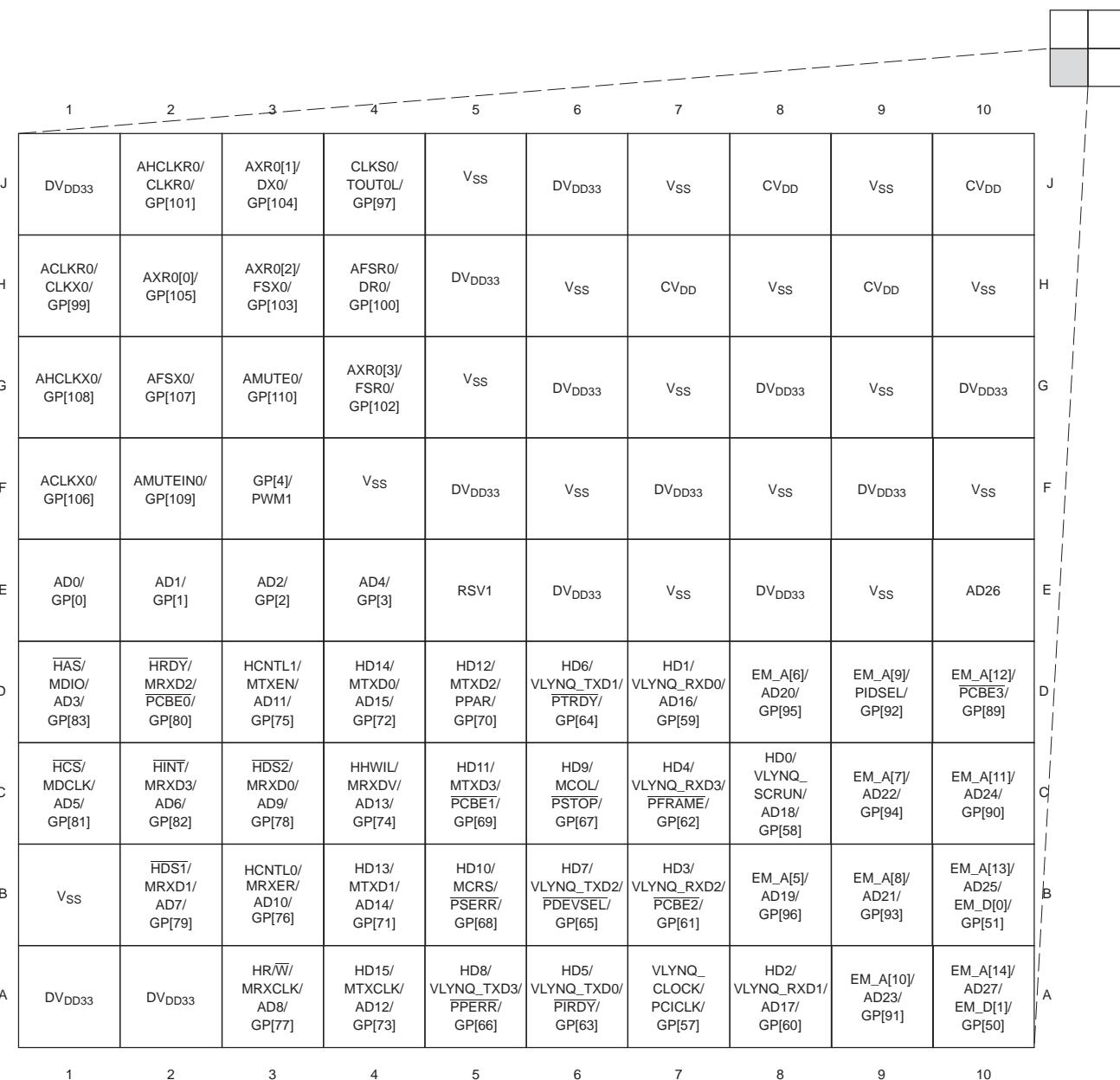
The diagram illustrates the ZWT Pin Map for Quadrant D, showing the connections for pins 1 through 10 across ten rows labeled J, H, G, F, E, D, C, B, and A. The connections are as follows:
