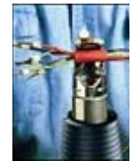
Applying Shrink Tubes
