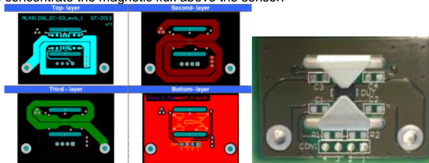
Figure 3: Low current applications with either multi-trace/multi-layer PCB (left) or closed shield (right).
