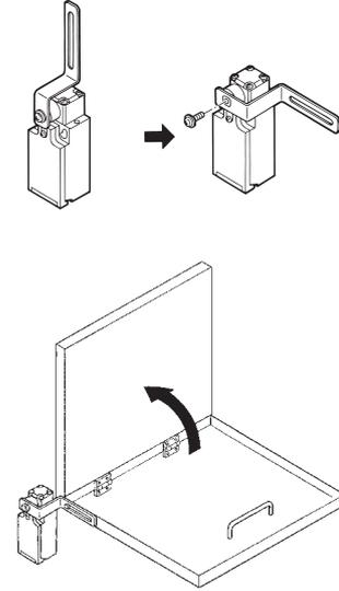
**Note:** Install the arm lever so that it will not rotate more than 180°.
