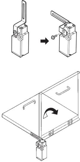
**Note:** Install the arm lever so that it will not rotate more than 180°.
