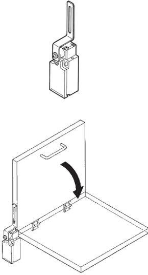
**Note:** Install the arm lever so that it will not rotate more than 90°.
