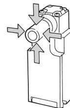
Be sure that the arm lever and door are mounted as shown in the following diagram so that the arm lever and head are not subjected to mechanical stress when the door opens or closes.
