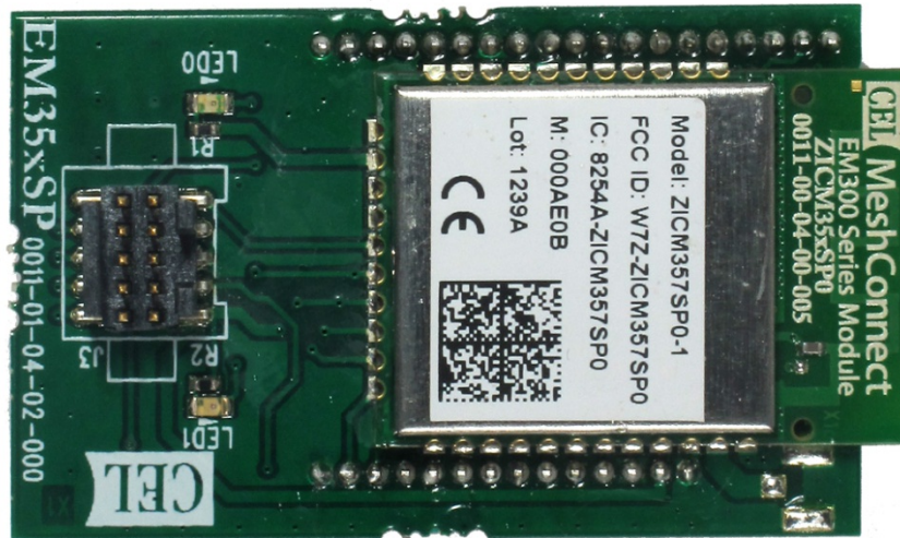
Figure 17. Module with PCB Antenna
