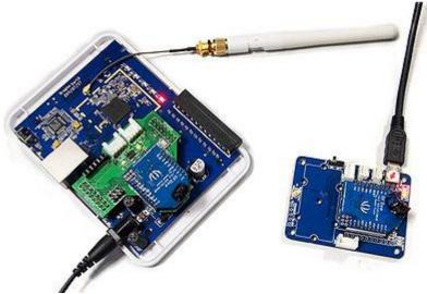
There are two RFbees used in this demo. One was inserted onto the Dragrove's XBee socket and the other was inserted onto an XBee Carrier. Set the baudrate to 9600.
