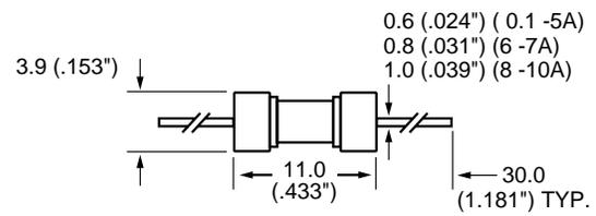
Axial Lead Material: Solder coated copper.
