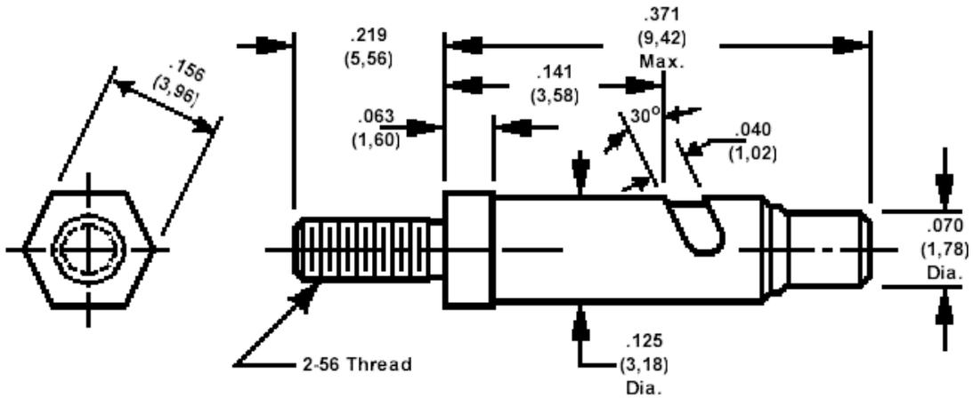
Recommended Lead Wire Sizes - #30 AWG (.010) (0,25) Min. Thru #22 AWG (.025) (0,64) Max.
