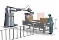
is performed. A limit switch or other means is used to detect when the robot is in a safe position and muting is then applied.
