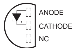
LP (TO-92/TO-226) PACKAGE (TOP VIEW)
