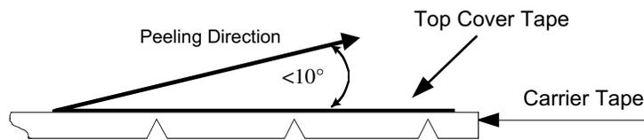
Peel-off force should be in the range of 0.1 – 0.6 N at a peel-off speed of  $300 \pm 10$  mm/min.
