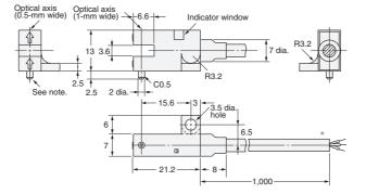
\* Vinyl-insulated round cable of 3.5 dia., 3 cores, (0.14 mm<sup>2</sup> with 1.0-dia. insulator); Standard length: 1 m
