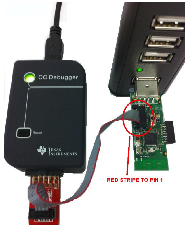
Figure 11 CC2540 USB Dongle Connected to CC Debugger
