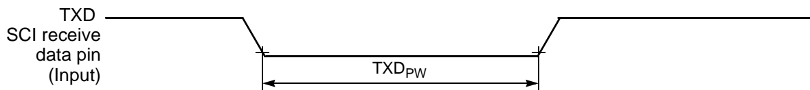
Figure 10-16 TXD Pulse Width
