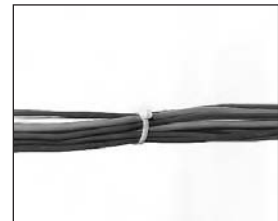
4. Finished tie holds cables firmly.
