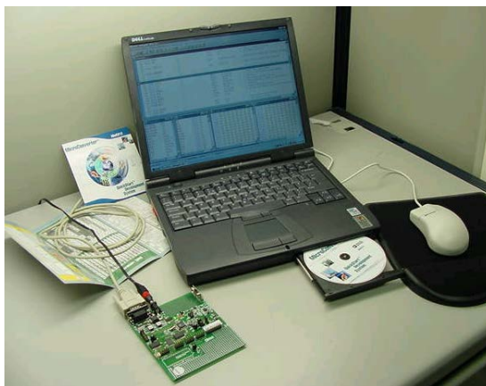
Figure 1. The ADuC8xx QuickStart Development System
