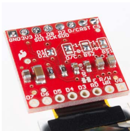
Breakout jumpers set for I 2 C mode.
