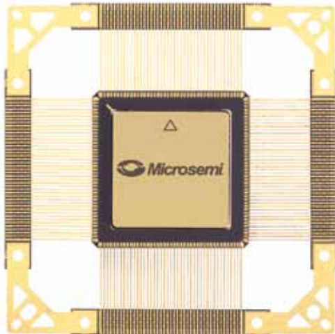
CQ172 b.s. 1.18x1.18" (29.972x29.972 mm) h. 105 mils (2.67 mm) p. 25 mils (0.64 mm)
