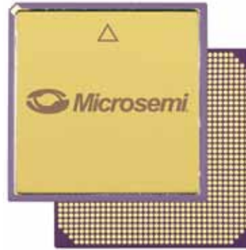
CG1272/LG1272 RTAX4000S and RTAX4000SL only b.s. 1.457x1.457" (37.00x37.00 mm) h. CCGA – 218 mils (5.535 mm) h. CLGA – 129 mils (3.28 mm) p. 39 mils (1.00 mm)
