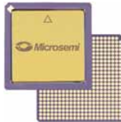
CG484/LG484 b.s. 0.91x0.91" (23.00x23.00 mm) h. CCGA – 225 mils (5.72 mm) h. LGA – 138 mils (3.51 mm) p. 7.5 mils (0.19 mm)
