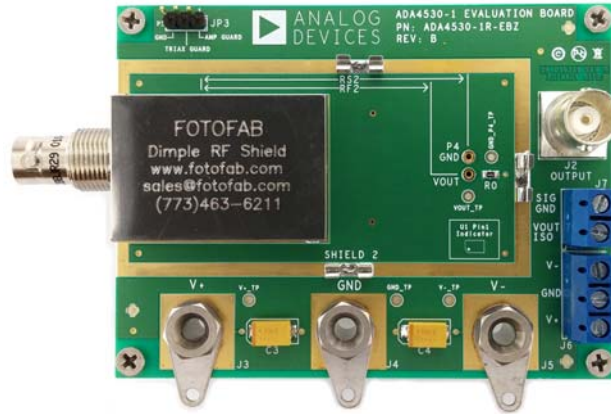
Figure 21. Evaluation Board Top View with SHIELD1
