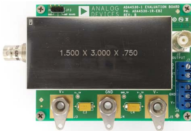
Figure 23. Evaluation Board Top View with SHIELD2
