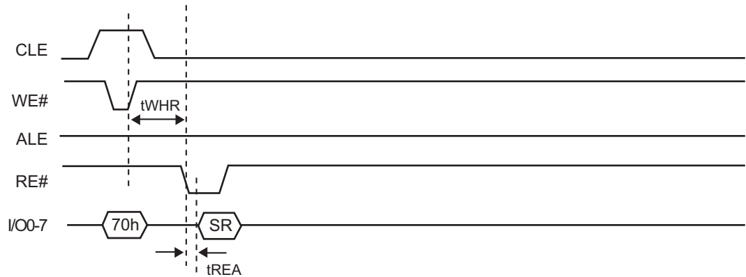
Figure 6.24 Read Status Timing
