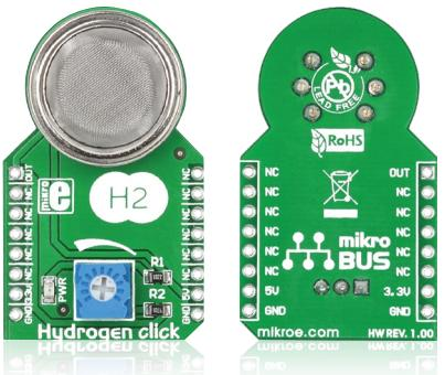
Hydrogen click™ is a simple solution for adding a high sensitivity hydrogen ( $H_2$ ) sensor to your design. It's suitable for designing gas leakage equipment. The board features an **MQ-8** sensor, a calibration potentiometer, a **mikroBUS™** socket and a power indicator LED. Hydrogen click™ communicates with the target board through mikroBUS™ AN (OUT) line. Hydrogen click™ is designed to use a 5V power supply only.
