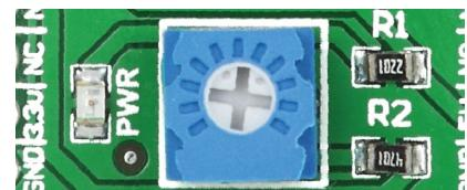
To calibrate hydrogen click™ for optimum performance, use the on-board potentiometer to adjust the load resistance of the sensor circuit.
