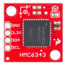
As you can see, the breakout has only four pins broken out. Two are for power, 3.3V and GND. Two are for I2C communication, SCL (clock) and SDA (data).
