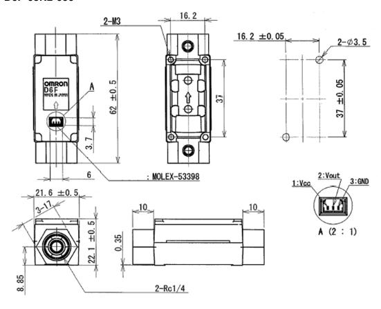
Note: Mount using an M3 pan head screw, tightened to 0.59 N•m max. torque.
