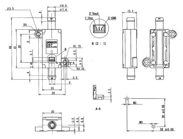
Note: Mount using an M3 pan head screw, tightened to 0.59 N•m max. torque.
