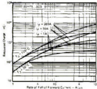
Fig. 34 – Typical Recovered Charge Vs. Rate of Fall of Forward Current, 85HFL\_S05 Series
