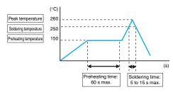
These conditions, however, depend on the type of solder, the manufacturer, the amount of solder, the size of the board, and the other mounting materials.
