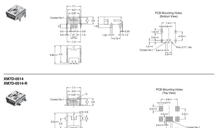
\* The adhesive tape is on the top surface of the Connectors.
