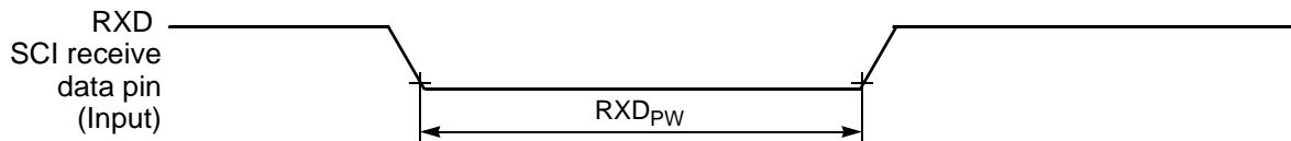
Figure 10-15 RXD Pulse Width
