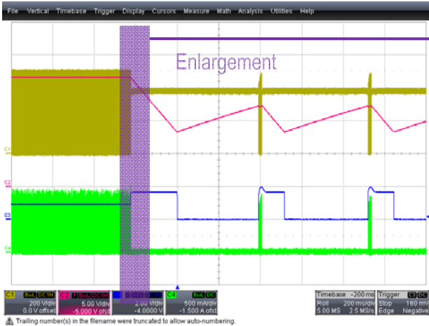
Figure 31. OSP Triggered: V_{FB} = 1.60V , 5V Output Short with 265V AC and Full-Load, CH1: V_{DS} (200V/div), CH2: V_{CC} (5V/div), CH3: V_{FB} (2V/div), CH4: I_{DS} (500mA/div), Time: 200ms/div and 10ms/div
