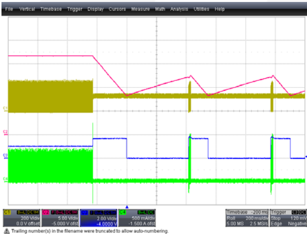
Figure 36. 5V Diode Short at 90V AC and Full Load Condition, CH1: V DS (200V/div), CH2: V CC (5V/div), CH3: V FB (2V/div), CH4: I DS (500mA/div), Time: 200ms/div
