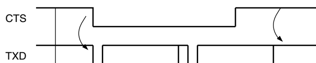
Figure 39-28. Transmitter Behavior when Operating with Hardware Handshaking
