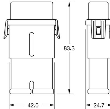
The In-Line Splash-water-proof fuseholder provides an efficient, simple installation method for MAXI / FK3-style fuse applications in harsh under-the-hood environments
